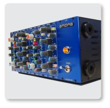
complete confidence. The included rackmount kit allows the L6 to be installed in standard 19" studio and touring racks. Designed to accommodate all 500 series-compatible modules and plug-in cards, the L6 is the perfect companion for your MICROPHONE PREAMPLIFIER 502, COMPRESSOR LIMITER 522, PARAMETRIC EQUALISER 512, and the many other modules currently under development – as well as those from 3rd party vendors.
